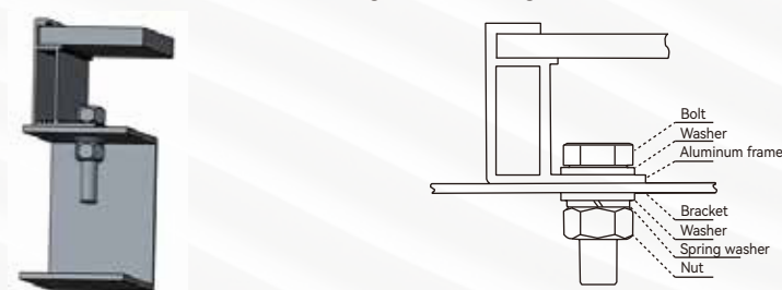
Figure 5 Bolt Installation of Mono-facial Modules
